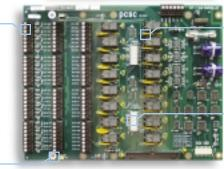
Integrated Self Resetting Poly-Switch Fuses in Series with Floor Relay Contacts. Eliminates Need for Series Wiring of External Fuse.
