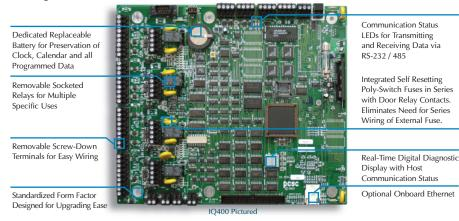
The **IQ Series** controllers are PCSC's benchmark for access control, input and output control monitoring. System configuration begins with either a two door controller (IQ 200) or a four door controller (IQ 400). Each controller can be expanded in 4 reader increments, up to 10 or 12 readers. Modular upgrades with add-on readers, inputs and outputs are engineered into the IQ Series design enabling you to dynamically configure a custom security system with standard off the shelf components.
